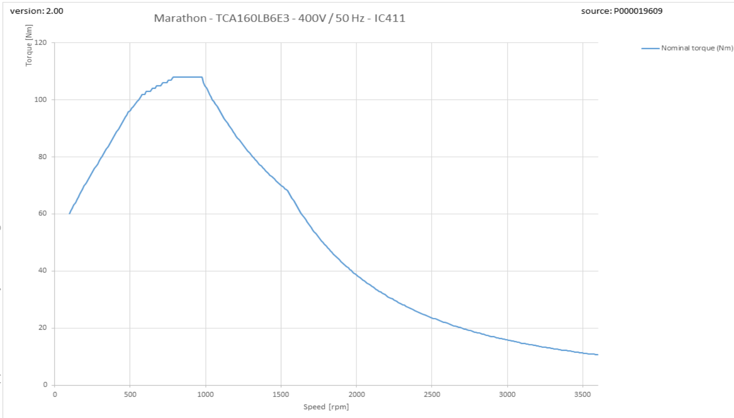
Torque versus Speed curve with variable frequency drive
